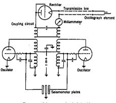
FIGURE 4.-Selamometer electrical circuit.
