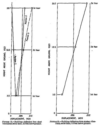
The translational fundamental frequencies were determined with the shaker. The north-south frequency was 5.8 cycles and the east-west frequency 7.0 cycles. There was a suggestion of torsional resonance, but it was not clearly defined.
