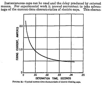
teristic is illustrated in figure 38, which indicates that the detonation of a cap may be delayed by decreasing the number of amperes of current passing through it. Figure 30 shows a circuit that permits con-
