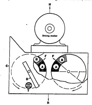
FIGURE 8.—Mechanical shaker: A, Fired weight; B, mayable weight; C, has for horizontal force; D, speed-phase bar; F, force; JI-H, ino of force; T, telephone earpices.
