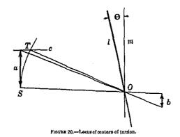
When two displacement recorders respond to vibrations along parallel lines, the locus of centers of torsion can be determined readily by the graphic method shown in figure 20. Assume the magnitude and direction of the recorded vibrations as represented by vectors a and b(fig. 20). Vector a is parallel to b; that is, the recorders have been
