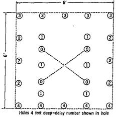
FIGURE 37 .- Hole arrangement for test shot (adit).
