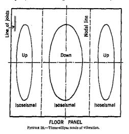
parallel the joists, showing that the panels have different elastic constants along the two major axes. The displacement at the center of the middle ellipse soon becomes maximum because the amplitudes of the outer ellipses drop as the frequency is raised and the amplitude of the center ellipse increases. As the two outer ellipses are out
