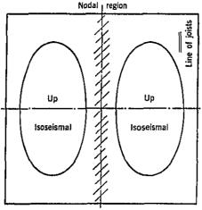
FIGURE 27.- Two-ellipse mode of vibration.
