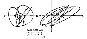
Figure 5.--Path of a vibrating point: A. Path of particle for 1 second resulting from a 13,400-pound shot 3,600 feet away; B, path of particle for the second following that in A.
