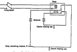
FITURE 39.-Delay firing circuit for two caps.
