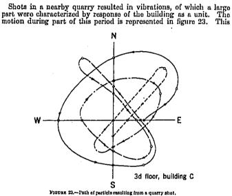
motion can be duplicated essentially by adding two horizontal vibra-tions that are acting simultaneously and are mutually perpendicular. The frequencies of the two vibrations correspond to the two fundamental translational frequencies, 5.8 and 7.0 cycles per second, and
